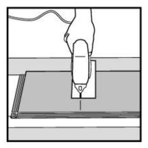
6. Second row, First plank minimum length of 1ft 7 11/16" (500mm). Leave an expansion gap of 3/8" (10mm) against the wall. Generally, the minimum distance between short ends of planks in parallel rows shall not be less than 6 inches (150mm).
