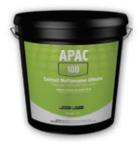
*APAC 100* contract multipurpose adhesive is a medium-solids, latex-based adhesive with good bond strength and rebond characteristics. *APAC 100* dries to a flexible, rubbery bond line that has good tack and rebond characteristics. Light in color, *APAC 100* is a good choice for the installation of basic carpet types and felt-backed vinyl sheet flooring in light commercial applications.
